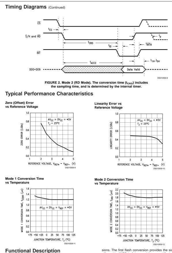
The ADC1061 digitizes an analog input signal to 10 bits accuracy by performing two lower-resolution "flash" conver-
