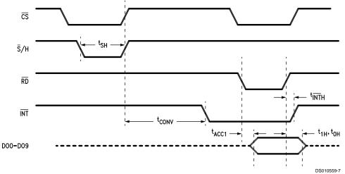
FIGURE 1. Mode 1. The conversion time ( $t_{\text{CONV}}$ ) is determined by the internal timer.
