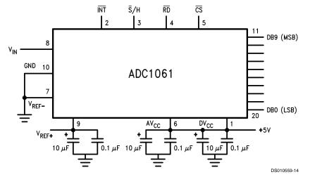
FIGURE 4. Typical connection. Note the multiple bypass capacitors on the reference and power supply pins. If  $V_{REF}$ - is not grounded, it should also be bypassed to ground using multiple capacitors (see 5.0 "Power Supply Considerations").
