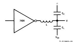
FIGURE 5. Clock Coupling
