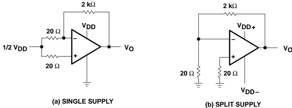
Figure 2. Noise-Test Circuit
