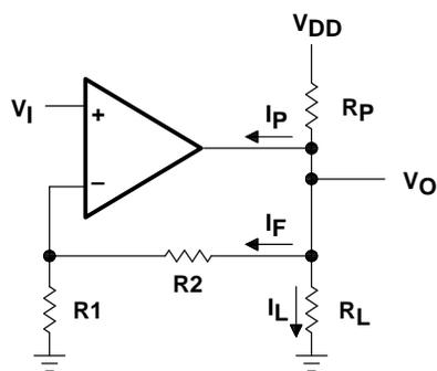
$$R_p = \frac{V_{DD} - V_O}{I_F + I_L + I_p}$$
