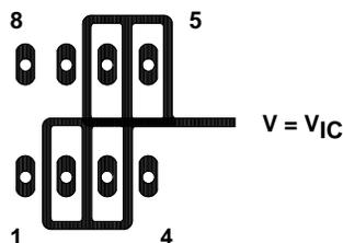
**Figure 4. Isolation Metal Around Device Inputs
