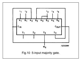
inputs are equally weighted. The outputs  $\Sigma$  0,  $\Sigma$ 1 and  $\Sigma$ 2 produce a binary number equal to the number inputs (I<sub>1</sub> to I<sub>5</sub>) that are HIGH. Figure 10 shows a method of implementing a 5-input majority gate. When three or more inputs (I<sub>1</sub> to I<sub>5</sub>) are HIGH, the output M<sub>5</sub> is HIGH.
