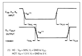
Fig.6 Waveforms showing the inputs ( $C_{IN}$ ,  $A_n$ ,  $B_n$ ) to the outputs ( $\Sigma_n$ ,  $C_{OUT}$ ) propagation delays and the output transition times.
