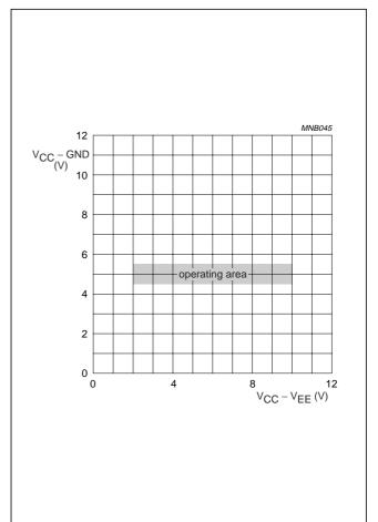
Fig.8 Guaranteed operating area as a function of the supply voltages for 74HCT4052.
