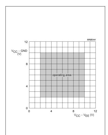
Fig.7 Guaranteed operating area as a function of the supply voltages for 74HC4052.
