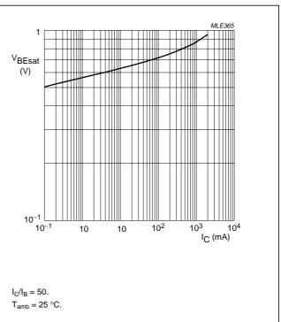
Fig.12 Base-emitter saturation voltage as a function of collector current; typical values.
