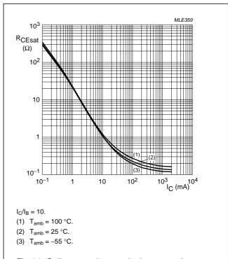
Fig.14 Collector-emitter equivalent on-resistance as a function of collector current; typical values.
