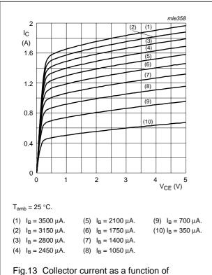
Fig.13 Collector current as a function of collector-emitter voltage; typical values.
