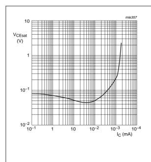
$I_C/I_B = 50$ .  $T_{amb} = 25 \,^{\circ}C$ .
