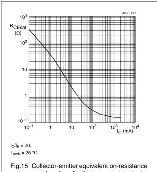
Fig.15 Collector-emitter equivalent on-resistance as a function of collector current; typical values.
