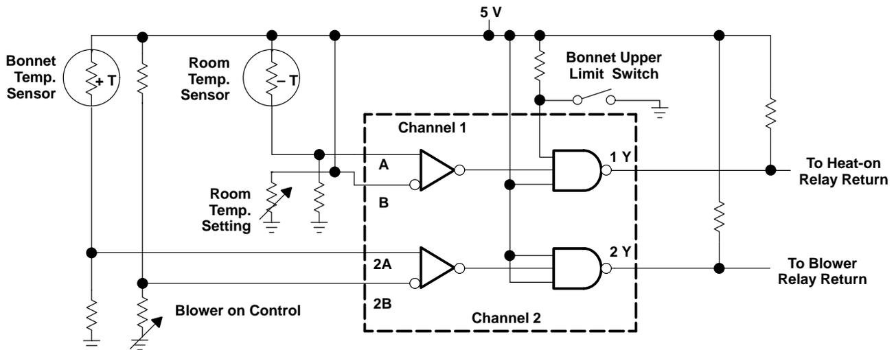
**Figure 18. Furnace Control Using SN55108A**
