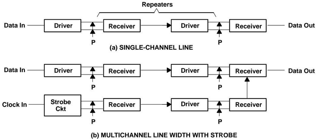
**Figure 19. Receiver-Driver Repeaters**
