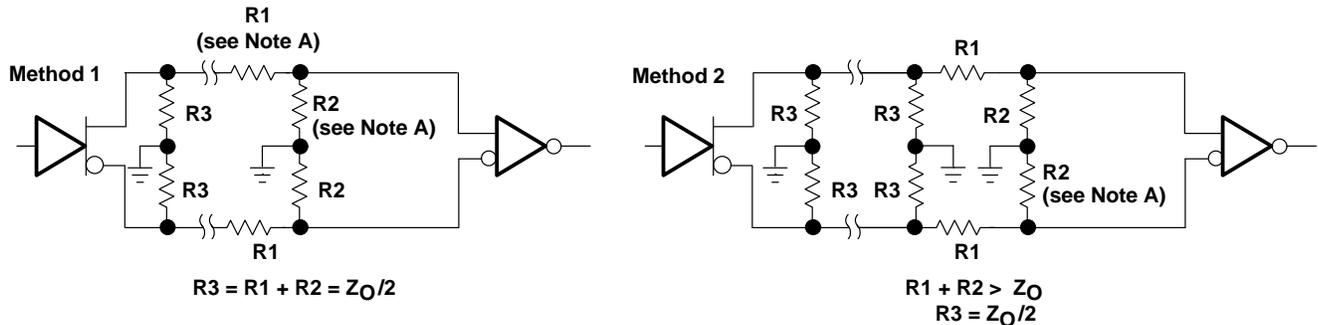
NOTE A: To minimize the loading, the values of R1 and R2 should be fairly large. Examples of possible values are shown in Table 1.
